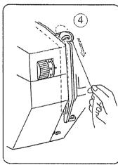
1. Draw thread through thread 2. While holding thread near 4. Draw thread up & through take-up lever.
